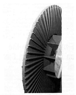
Fig. 2 The left-hand disk showing the fins and central vanes
